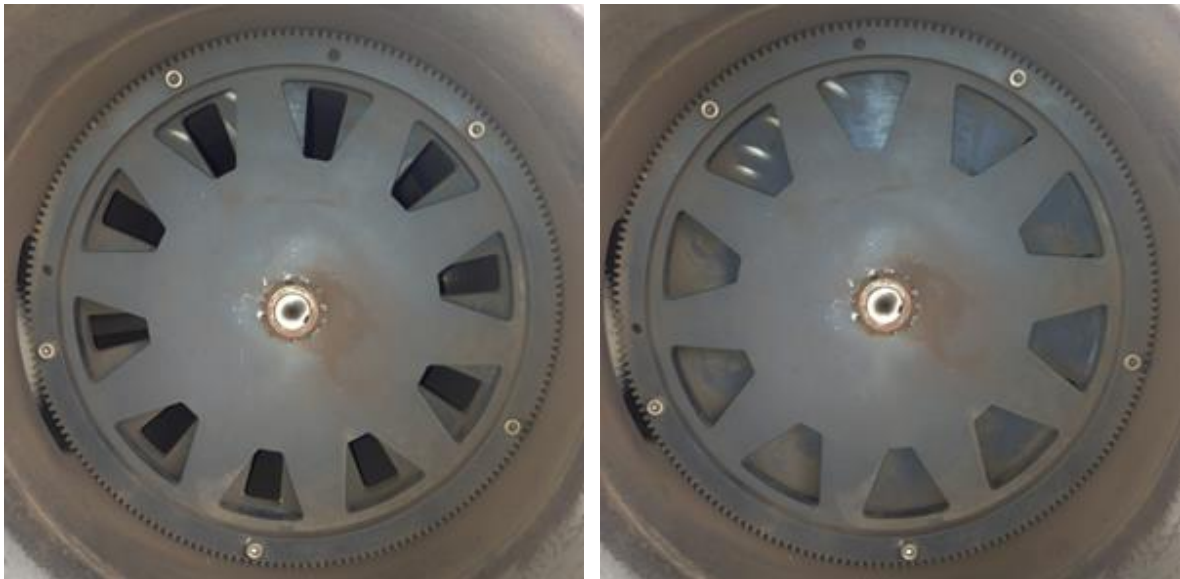
Figure 22. The pulsation generator rotor and stator plates showing open and closed
