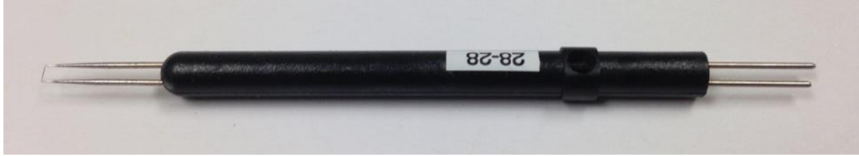
Figure 27. Hot-wire anemometer tip (Model 1201 - TSI, Inc.)
