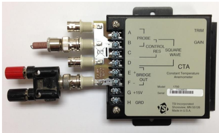
Figure 26. Hot-wire anemometer bridge circuit (Model 1750 - TSI, Inc.)
